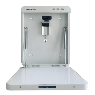
The box is made of cold-rolled steel, with four arc-shaped corners and no sharp angles, which is anti-collision and effectively improves the safety of use; it has built-in handles for easy opening of the equipment; 20mm pure aluminum alloy display board can place heavy books and can bear up to 5KG; The board is supported by two metal pneumatic rods with a diameter of 10mm, which is reliable and strong; the built-in chassis lock is safe against theft and damage;
